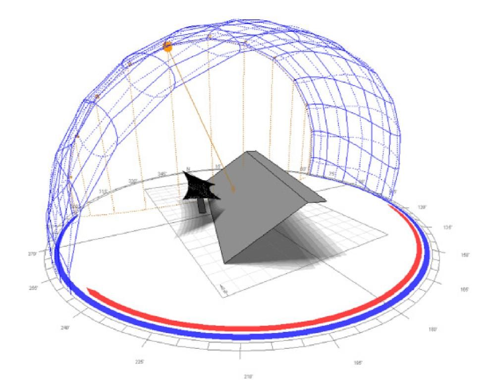
Figure 38. Three-dimensional solar sun path diagram with hourly shade projection. Source: (Image) elaborated by the authors.
