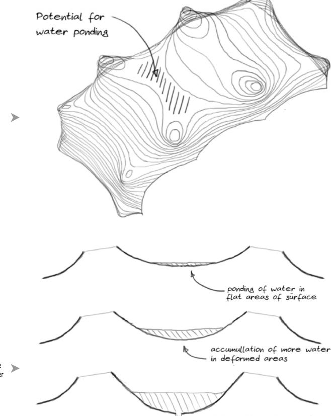
Figure 26. Analysis of drainage and potential areas for water ponding on a membrane structure with multiple high-points. Source: (Image) elaborated by the authors.
