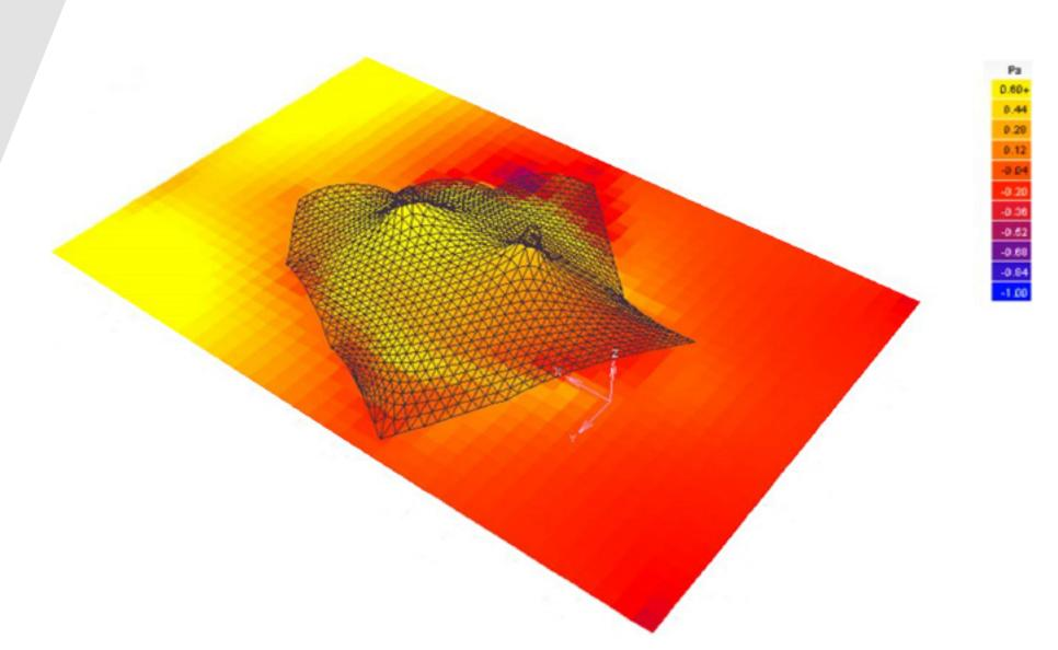
Figure 36. CFD airflow analysis showing air pressure at membrane height in perspective-view.
