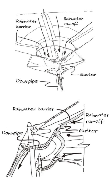
Figure 29. Draining barrier for borders and edges of the membrane. Source: (Image) elaborated by the authors.
