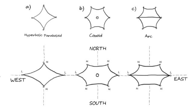
Figure 4. Solar orientation and proportion of membrane structures (plan-view), a) hyperbolic-paraboloid, b) conoid, c) arc. Source: (Image) elaborated by the authors.
