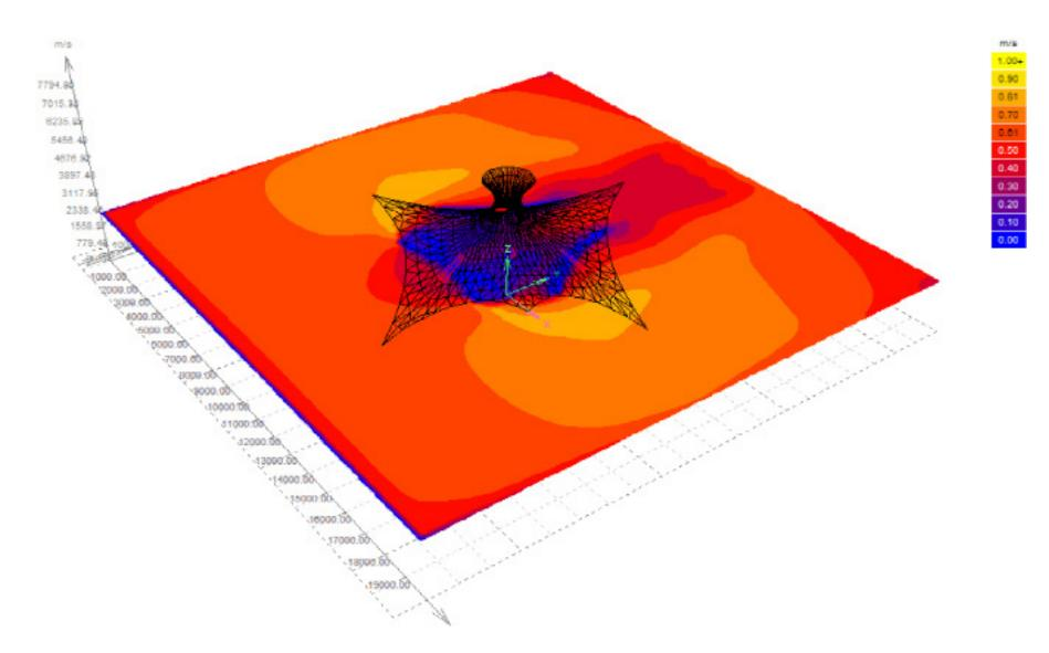
Figure 43. CFD análisis showing air velocity at membrane height (perspective view). Source: (Image) elaborated by the authors.
