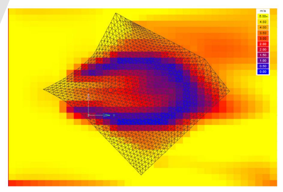
Figure 33. CFD airflow analysis showing air velocity membrane height in plan-view. Source: (Image) elaborated by the authors.
