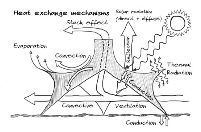
Figure 13. Heat exchange mechanisms on semiopen conoidal membrane structure.\* \*Note: The size of the arrows is not representative for the magnitude of the heat exchange. Source: (Image) elaborated by the authors.
