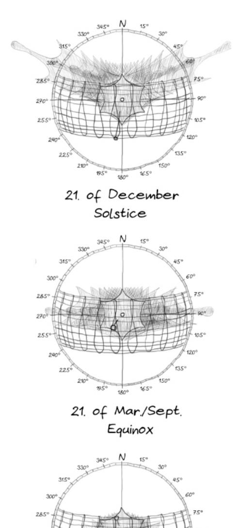
Figure 6. Solar charts with overlapping annual shade projection for conoidal membrane structure. Source: (Image) elaborated by the authors.
