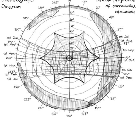
Figure 7. Shadow mapping of surrounding elements. Source: (Image) elaborated by the authors.
