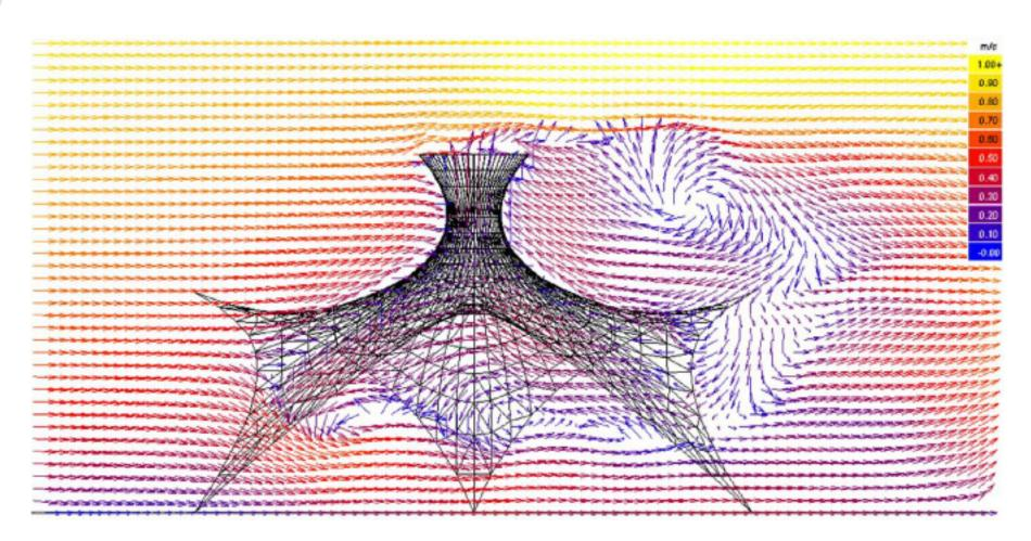
Figure 42. CFD analysis Air flow vectors and velocity (section view). Source: (Image) elaborated by the authors.
