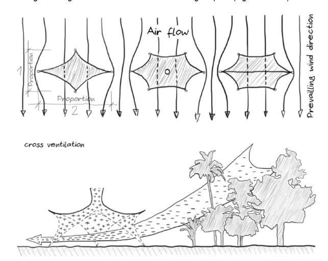
Figure 24. Cooling effect of surrounding vegetation in combination with cross-ventilation. Source: (Image) elaborated by the authors.
