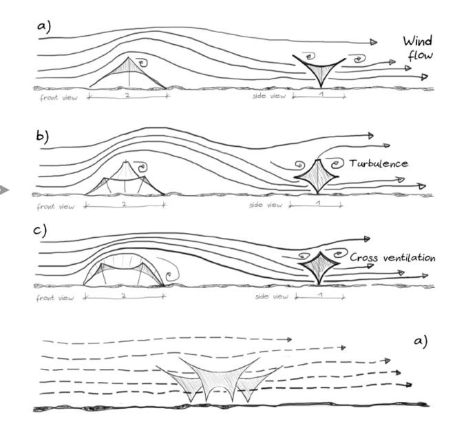
Figure 16. Aerodynamic effects on different membrane geometries: a) hyperbolicparaboloid, b) conoid, c) arc. Source: (Image) elaborated by the authors.
