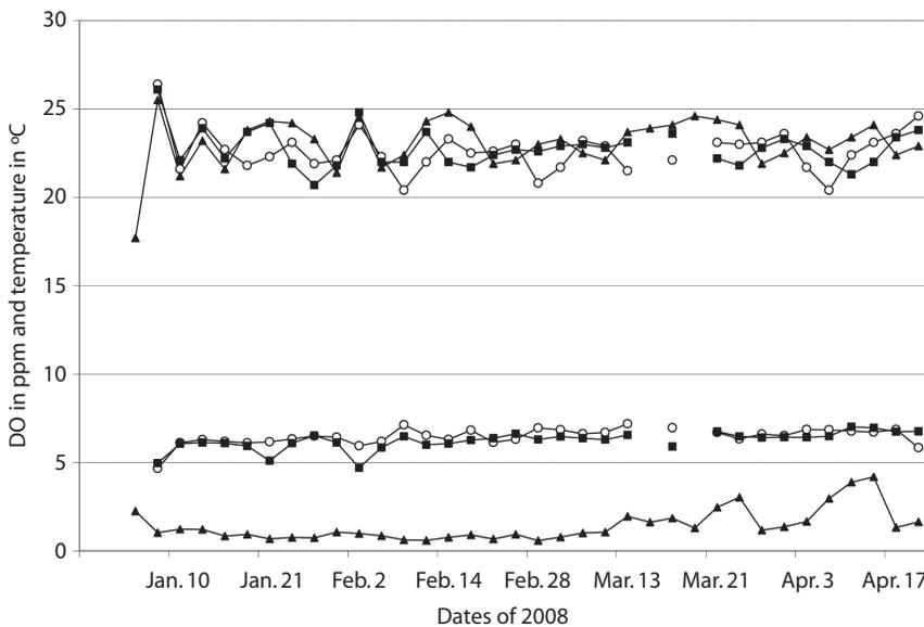
Fig. 1. Water temperature in  $^{\circ}\text{C}$  (above) and DO in ppm (below) in hypoxic and oxygenated water treatments in Experiment 2. (Circles=water regularly changed; squares=oxygenated wastewater; triangles=hypoxic wastewater).
