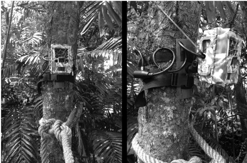
Fig. 3. Front and side view of the PC800 Hyperfire Professional Semi-Covert Camera trap mounted above a rope bridge.
