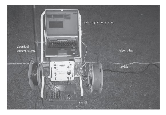
Fig. 3: Multi-electrode system used for 2- dimensional resistivity survey.
