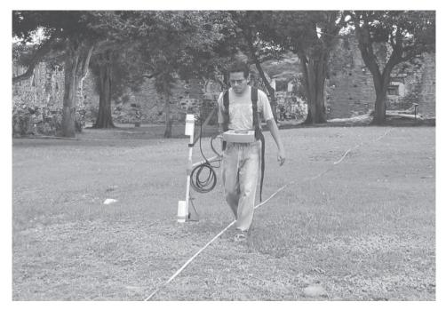
Fig. 2: Caesium magnetometer system (G-858 of Geometrics) in gradiometer mode.
