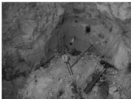
Fig. 14: Measurement of moisture content in TBJ slope (TMS1, left side of photo) and suction (tensiometer, right side of photo).
